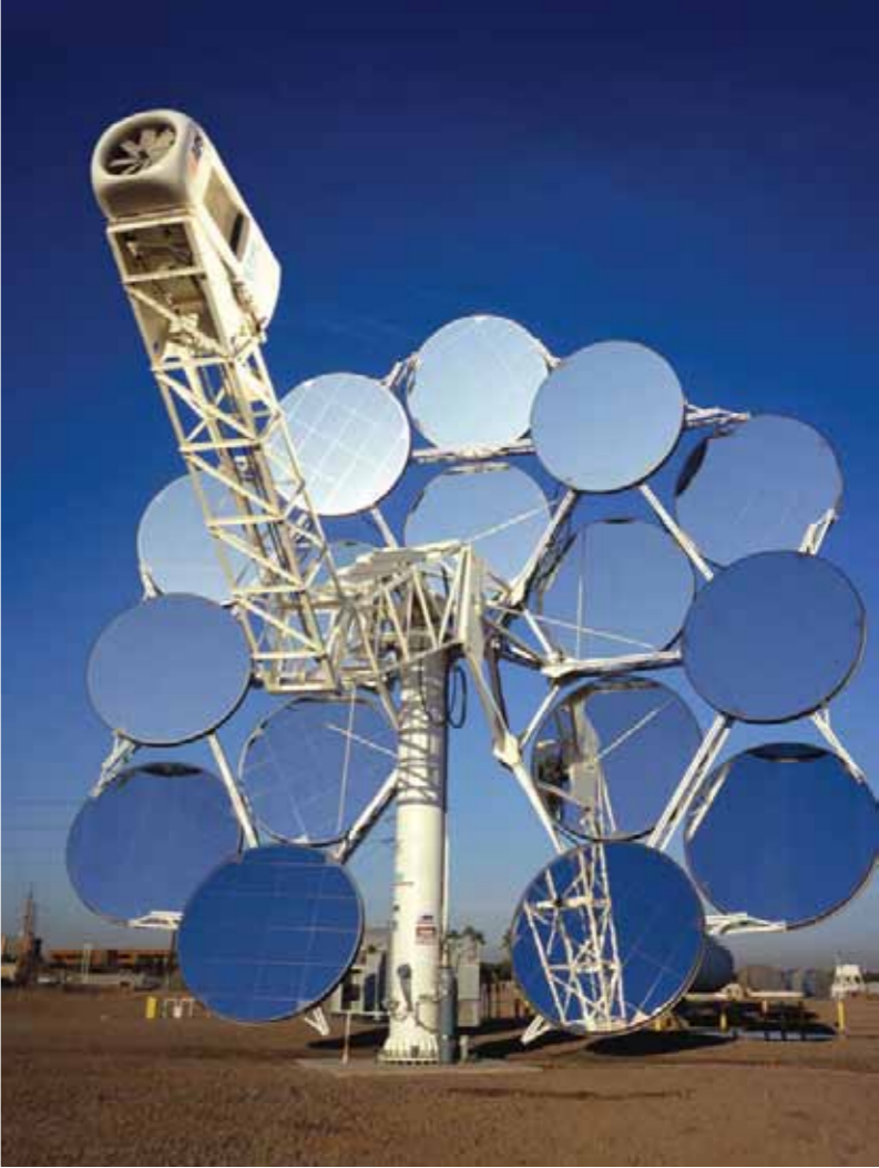
A Dish Stirling Solar power system is being tested at the Solar Test and Research Center in Tempe, Arizona. Its mirrors focus sunlight onto a thermal receiver, where a Stirling heat engine drives a generator producing 25 kilowatts of electricity.
